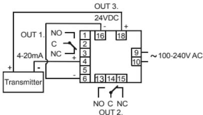
3-wire voltage output transmitter, power supply for transmitter, 1 relay output, 1 analogue output.
