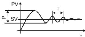
Record the Peak-to-Peak variation (P) of the first cycle (i.e. the difference between the highest value of the first overshoot and the lowest value of the first undershoot), and the time period of the oscillation (T) in minutes:
