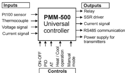
The RS485 Modbus RTU serial output provides digital communication interface with PC and remote programming possibility.
