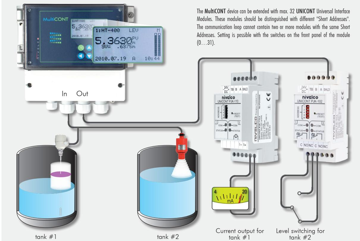
The MultiCONT device can be extended with max. 32 UNICONT Universal Interface Modules. These modules should be distinguished with different "Short Addresses". The communication loop cannot contain two or more modules with the same Short Addresses. Setting is possible with the switches on the front panel of the module (0...31).
