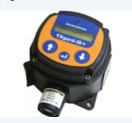
TXgard-IS+ is an Intrinsically Safe (I.S.), 2-wire, toxic and oxygen gas detector with local LCD display. A wide choice of sensors is available for use in a variety of applications. TXgard-IS+ is ATEX and IECEx certified for use in Zone 0,1 or 2 hazardous areas, and also UL and cUL certified for use in Division 1 or 2 hazardous areas.
