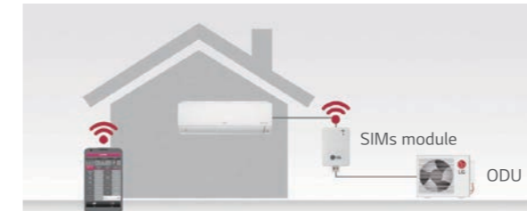
* SIMs : Smart Inverter Monitoring System
