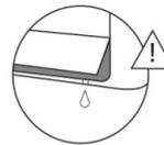
Caution: Do not keep louver at too vertical an angle for long periods of time. This can cause water condensation to drip on your furnishings.
