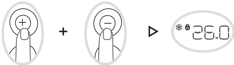
Press button “+” and “-” simultaneously for one second to activate LOCK function.
