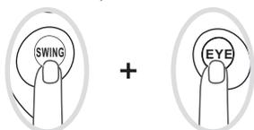
Press button “SWING” and “EYE” simultaneously for one second to turn the Electrical heating function on or off. A symbol
