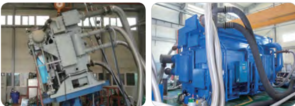
▲ High COP Single Effect 2-Lift Hot Water Driven Absorption Chiller
